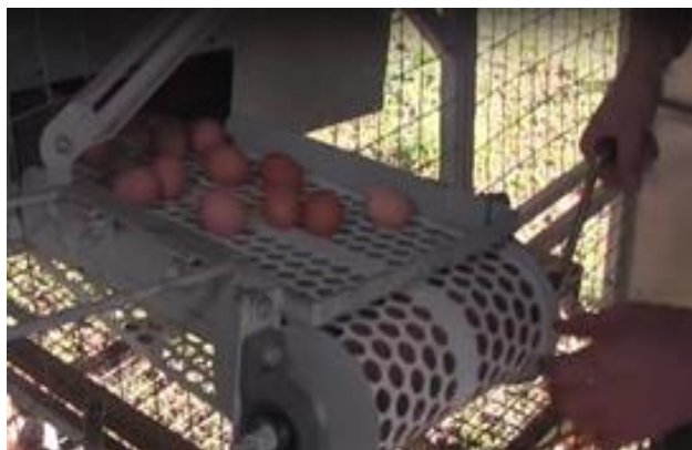
Fig. 5. Conveyor belt in a mobile hen house to collect eggs.
